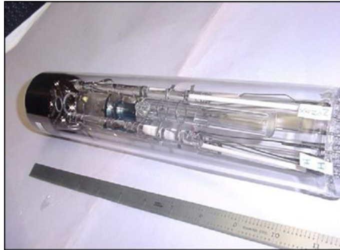
Figure 2. Test vehicle for xenon discharge testing of hollow cathodes.
