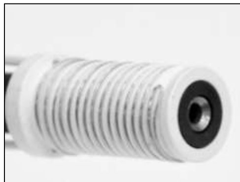
Figure 1. Double-helical rhenium heater filament wrapped around boron nitride cylinder. Heater shown above is installed in a hollow cathode assembly with the exterior sleeve removed.
