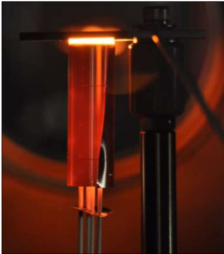
Figure 4. Complete close-spaced diode assembly operating at 980°C cathode temperature with a C12A7 emitter sample. The entire assembly runs inside the Plasma Test Facility.
