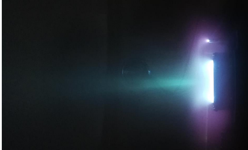
Figure 11. the photograph of HEP-140MF thruster discharge
