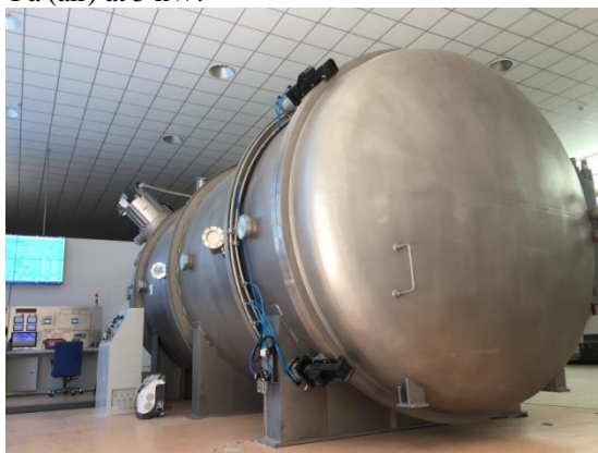
Figure 8. EPTS-2 electric propulsion test system
