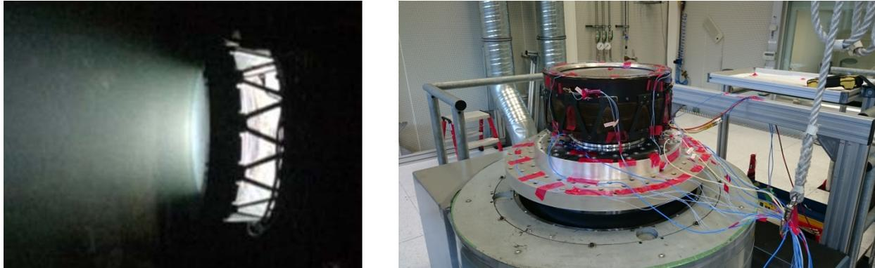
Figure 2 RIT 2X thruster firing (left) and RIT 2X thruster at the shaker (right)
