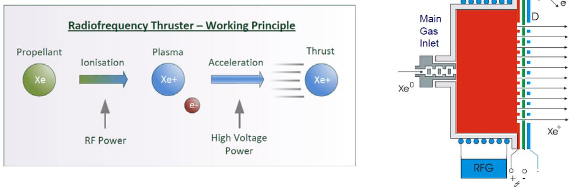
Figure 1 RIT Function Principle
