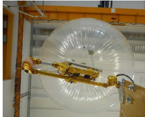
**Figure 6. Engineering Model 2 during deployment rehearsal.**
