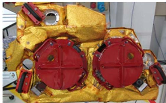
**Figure 3. Front view of the PTM with two SPT-140D thrusters.**
