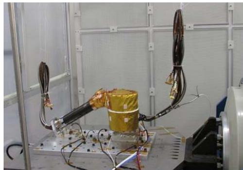
**Figure 7. Qualification Model during vibration tests.**
