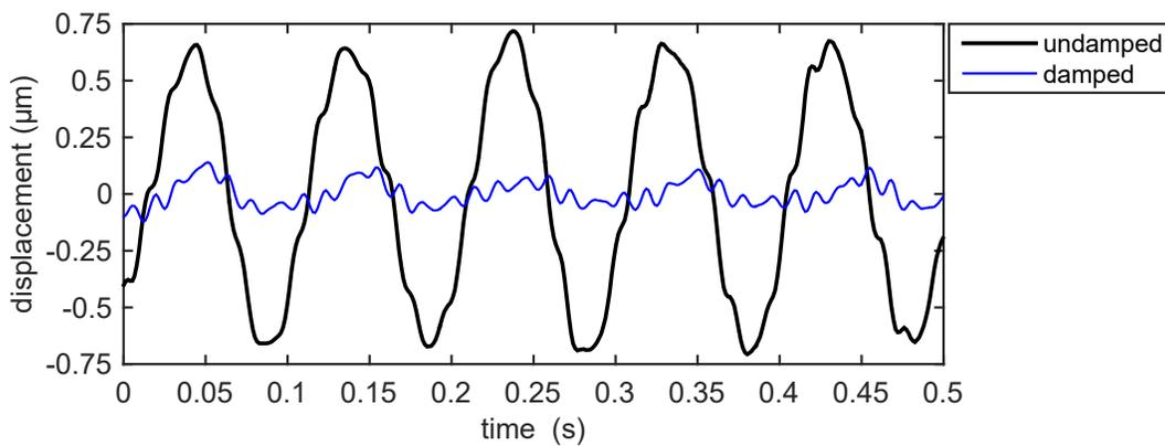
Figure 3. Mechanical noise. The time series show the recorded oscillations of the mirror (a) without and (b) with the eddy current damping unit. The measurement is performed in a common lab environment without further provisions for vibration absorption.
