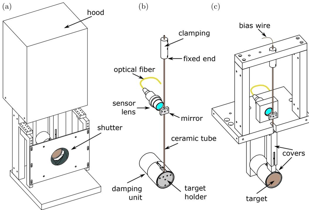
**Figure 1. Implementation of the force probe. (a) Probe with the optional shutter and the protective hood, (b) all essential parts of the probe, (c) necessary mechanical structures of the setup.**
