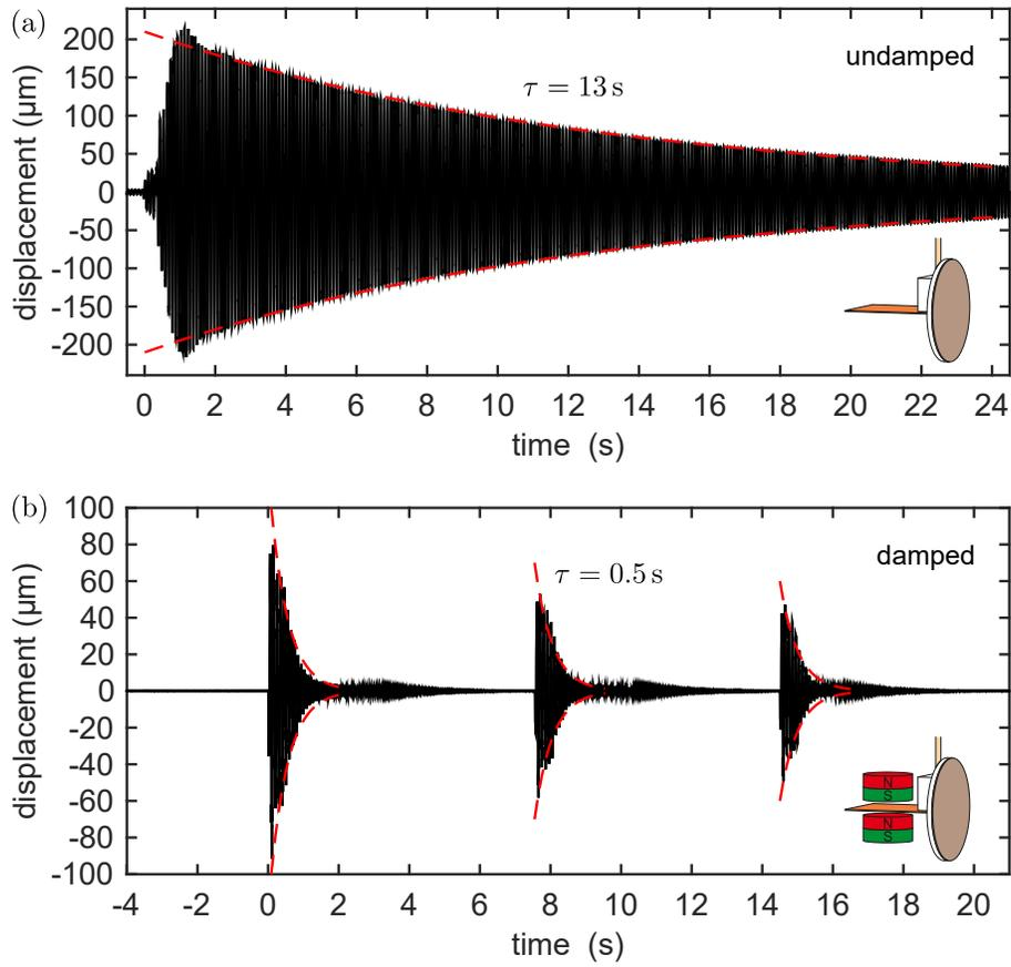
Figure 4. Decay of the oscillations caused by mechanical shocks, (a) without and (b) with the eddy current damping unit. The damping time constant  $\tau$  is significantly reduced by the damping mechanism.
