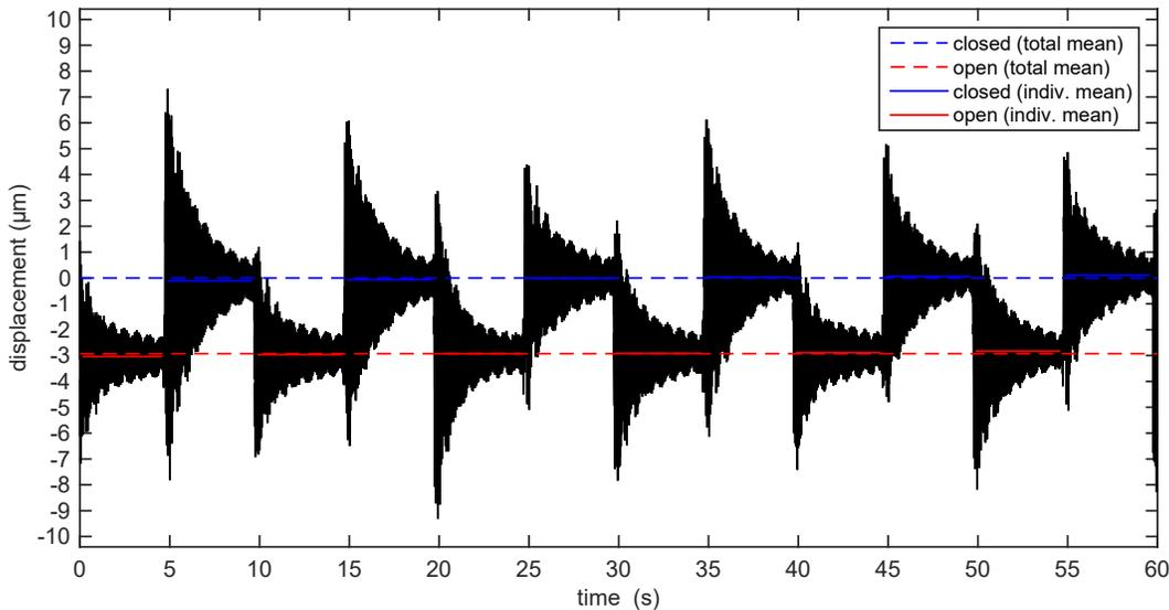
**Figure 6.** Time series of the measured displacements using the beam shutter. The forces are generated by a 1.2 keV Ar beam from a broad beam ion source. The probe is equipped with a carbon fiber velvet target with an area of  $A = 3.14 \text{ cm}^2$ . The red and blue dashed and solid lines indicate time averages corresponding to the intervals over which they extend.
