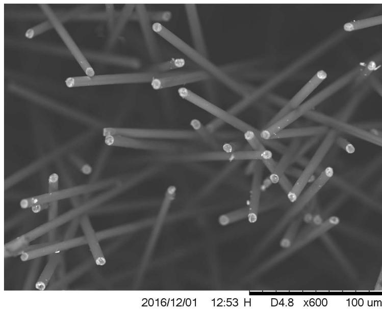
Figure 5. Scanning electron microscopy image of the carbon fiber velvet.
