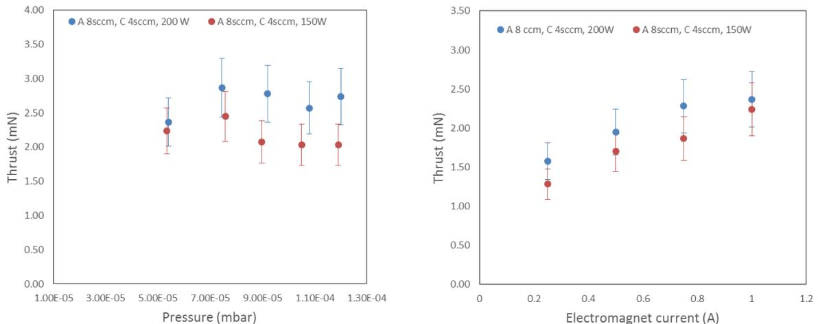
**Figure 7. Thrust as a function of the background pressure (on the left) and of the magnetic field (on the right) for different anode power levels.**
