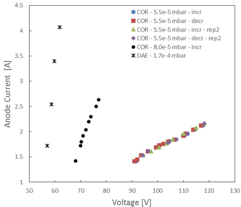
Figure 4. Voltage-current characteristics of the QCT operated in the Daedalus chamber at SSC and Corona chamber at EPL under different background pressure conditions.
