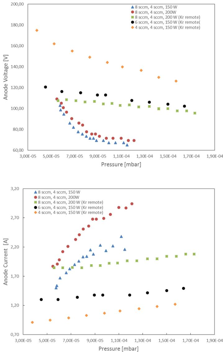
**Figure 5. Anode current and voltage as a function of the background pressure.**
