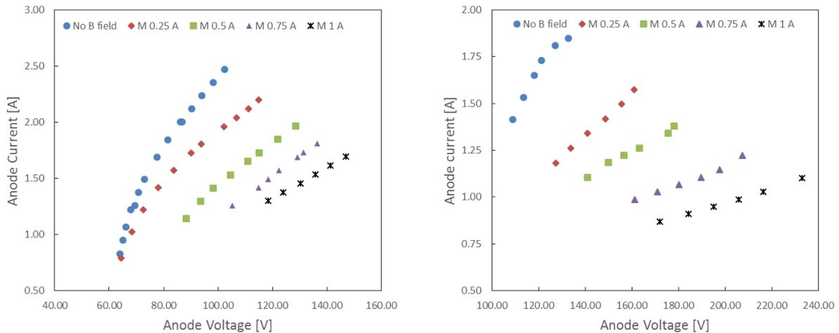
**Figure 6. Voltage-current characteristics of the QCT operated in EPL-Corona chamber applying different magnetic field levels for two different anode mass flow conditions. On the left 8 sccm, on the right 6 sccm. Cathode flow is 4 sccm in both cases.**
