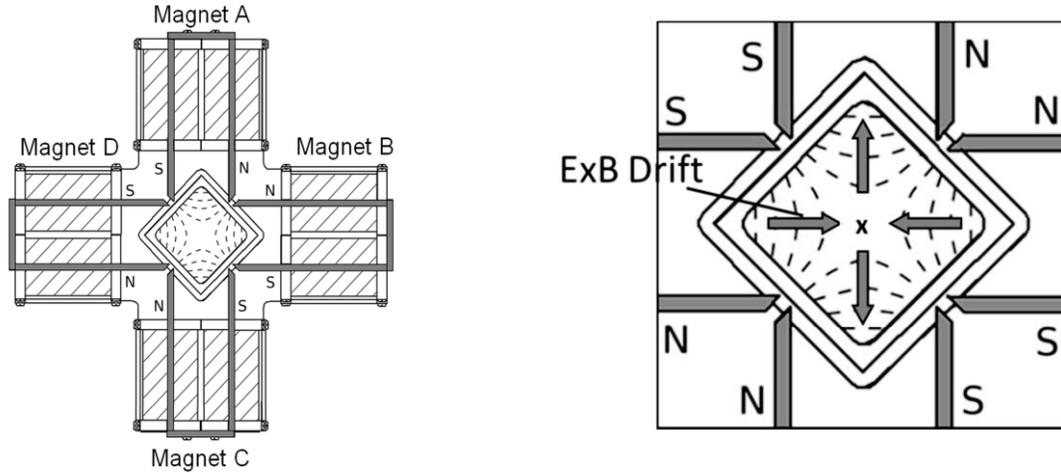
Figure 2. QCT magnetic field topology<sup>3</sup>.
