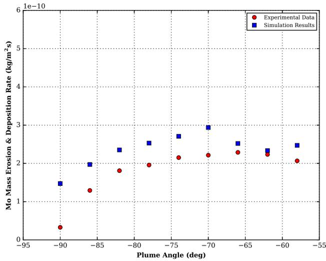
Figure 10. Net mass deposition rate for TL12 after splitting the Mo mass flow rate between two different particle injection algorithms.
