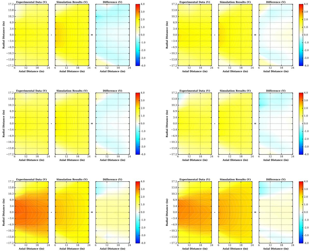
Figure 6. Plasma potential comparisons for TL1, TL5, TL9, TL12, TL19 and TL37 (thrust level contours are organized form left to right and top to bottom, respectively).
