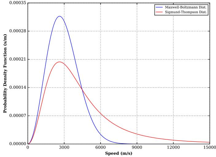
Figure 3. Maxwell-Boltzmann vs. Sigmund-Thompson velocity distributions.
