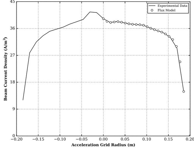
Figure 2. Beam current density versus radial distance at 3 cm for TL37.
