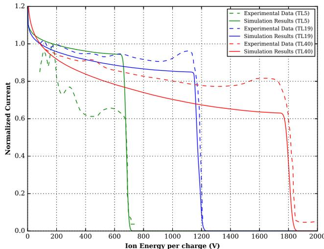
Figure 5. RPA data at 1 m distance and 45 deg plume angle for TL5, TL19 and TL40.
