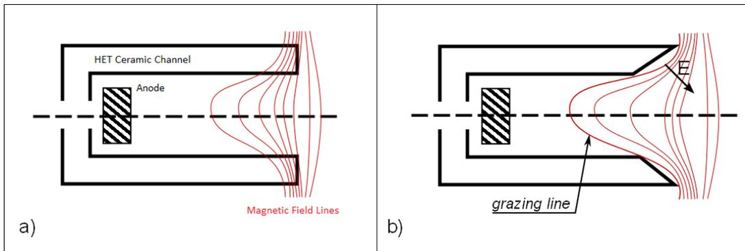
Figure 1. Magnetic field topologies for a standard HET (a) and for a magnetically shielded HET (b).
