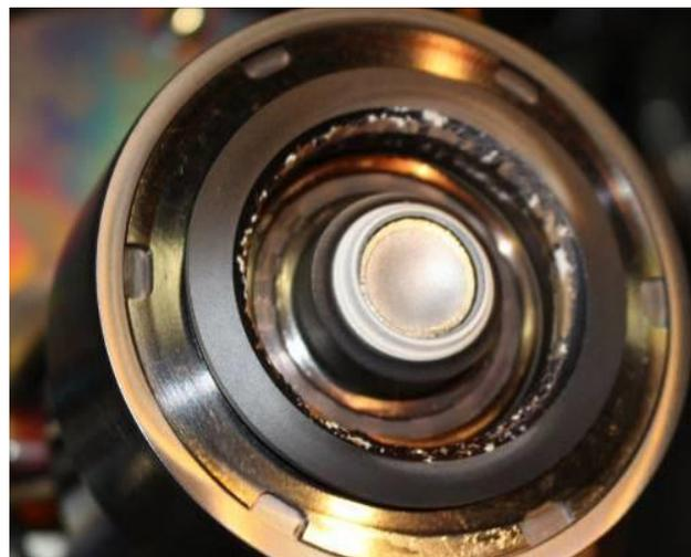
**Figure 7. MSHT100: post-test inspection after 350 hours of operation.**
