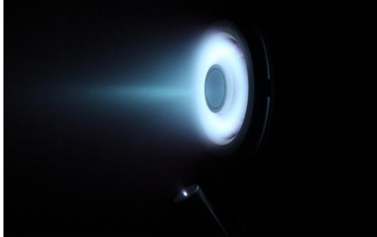
Figure 2. Magnetically shielded HT100 firing at SITAEL premises.
