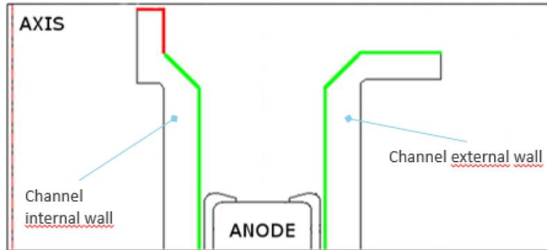
**Figure 6. MSHT100 ceramic walls: the magnetically shielded areas are marked with a green line, whereas the red lines identify the unprotected areas.**
