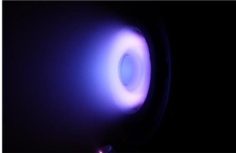
**Figure 8. MSHT100 firing with krypton.**
