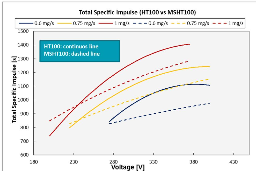
Figure 5. Comparison of total specific impulse-voltage curves for HT100 and MSHT100, at different Xe mass flow rates.
