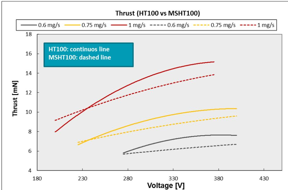
Figure 4. Comparison of thrust-voltage curves for HT100 and MSHT100, at different Xe mass flow rates.
