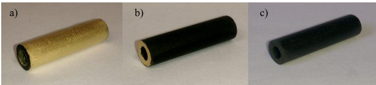
Figure 4. Gold coating on the surface of the insert. Three different kinds of gold-coated inserts have been available for testing. a) The gold is coated at the lateral surface of the insert tube, b) the gold is coated at the front side of the insert tube, c) reference insert with no gold coating at all
