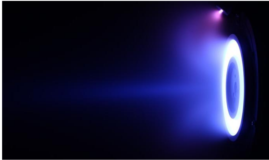
Figure 1. Thruster firing with pure krypton during the second PVT campaign.
