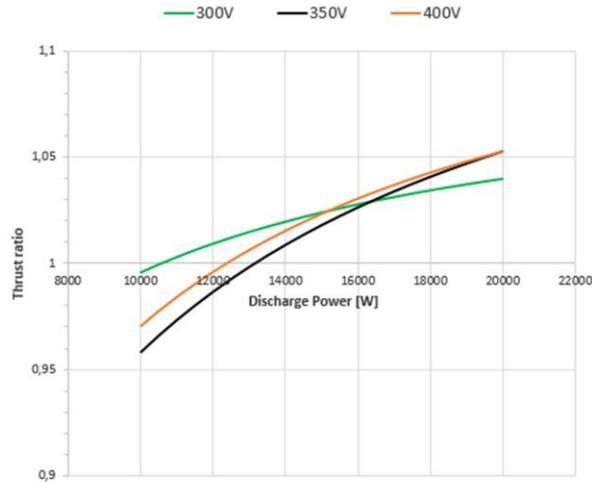
**Figure 8 Comparison of the HT20k between the first and the second campaign with the central cathode at various discharge voltages. The ratio is made on the measured thrust between second and the first campaign.**
