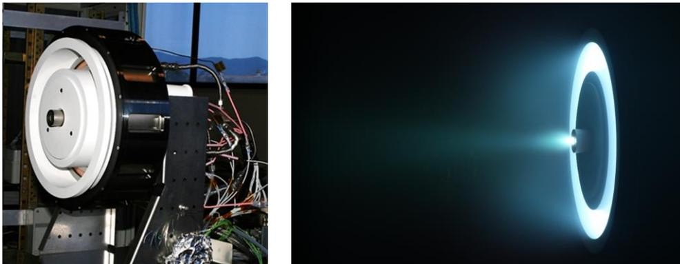
**Figure 5** HT20k mounted on the thrust stand for the first campaign (left), firing during characterization (right).
