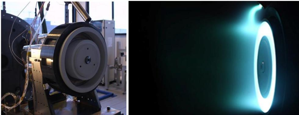
**Figure 7 HT20k mounted on the thrust stand for the second campaign (left) and firing at 300 V and 15 kW during the 150 hours test (right).**
