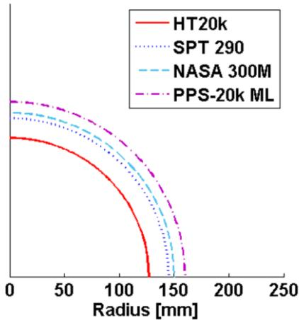
**Figure 1 Outer channel radius comparison for various 20 kW-class Hall thrusters.**
