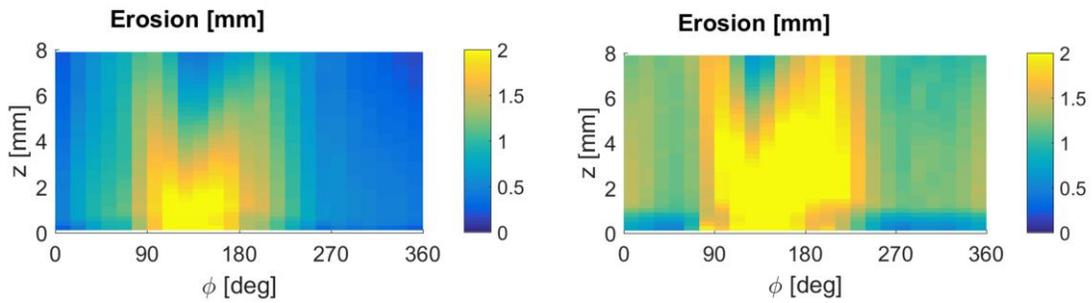
**Figure 10 Erosion of the inner (left) and outer (right) ceramic for the HT20k after 150 hours at 300 V and 15 kW with external cathode.**
