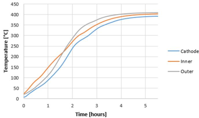
**Figure 6 Thermal transient of the HT20k at 400 V and 20 kW.**
