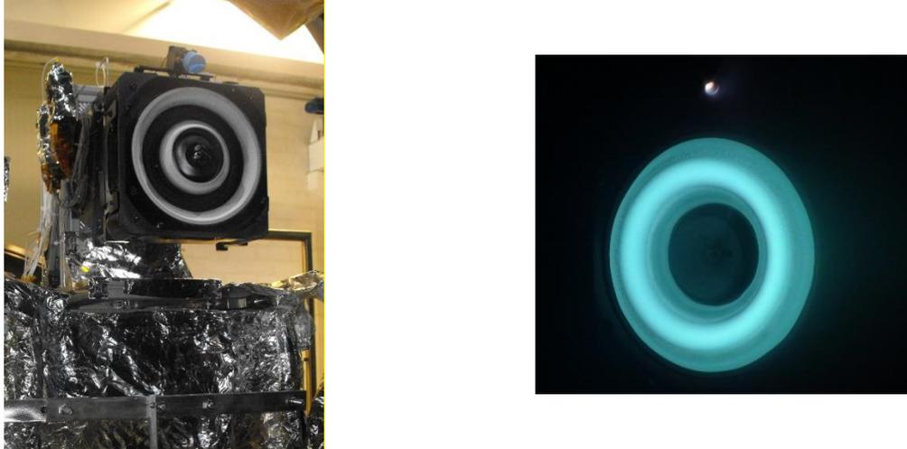
**Figure 2 – The PPS@5000 EM Hall Effect Thruster on the thrust balance in the LVTF2 facility.**
