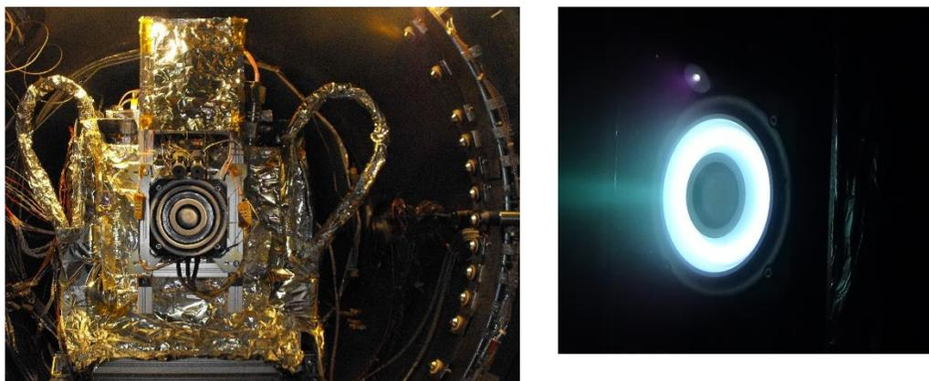
Figure 1 – The PPS@1350 Hall Effect Thruster on the thrust balance in the MVTF1E facility.
