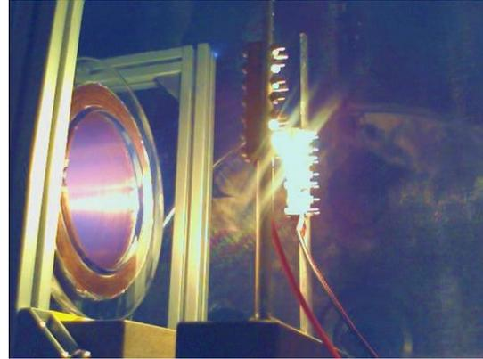
Figure 7. Electron bombardment ion thruster.
