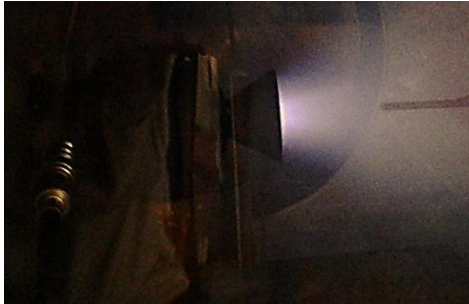
Figure 2. The HPH.Com thruster firing inside CISAS vacuum chamber. The tip of a Faraday probe immersed in the plume is visible on the right of the picture.
