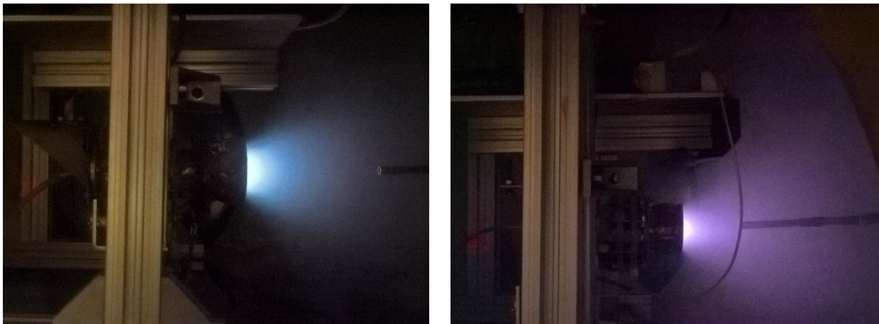
Figure 5. MHT testing with Xe (left) and Ar (right) propellants. The thruster is mounted in the thrust balance, while the Faraday probe is being employed for current measurements within the plume.
