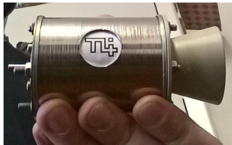
Figure 4. The MHT, held in hand by T4i personnel. The discharge chamber, RF antenna and magnets are enclosed within an EM shield structure. The small scale of the device can readily be appreciated.
