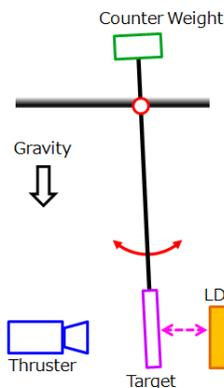
Figure.3 Target thrust stand
