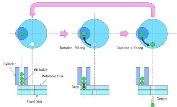
Figure.7 Method of  $\Delta M$  calibration
