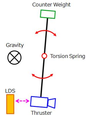
Figure.4 Torsion balance thrust stand
