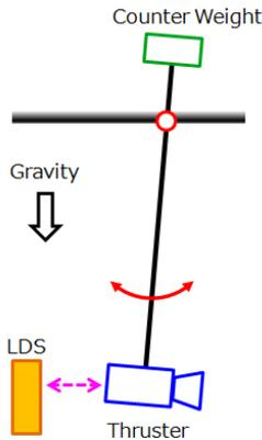
Figure.2 Pendulum thrust stand
