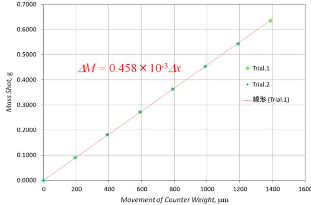
Figure.9 Result of  $\Delta M$  calibration
