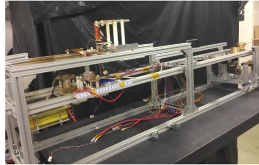
Figure.6 Seesaw type thrust stand
