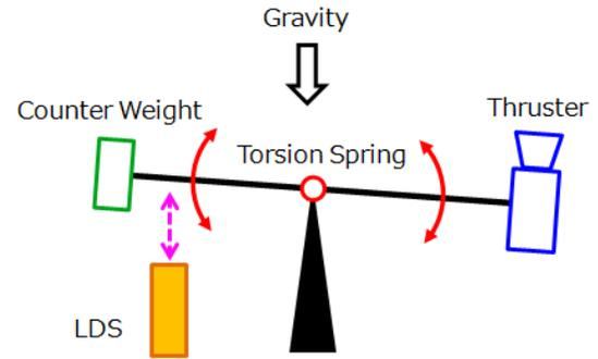
Figure.5 Schematic of seesaw type thrust stand
