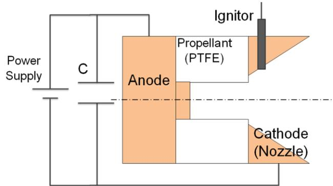
Figure.1 Electrothermal PPT
