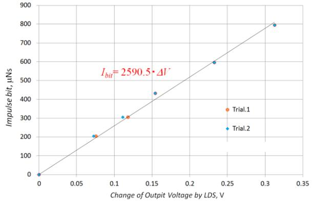
**Figure.11** Relation between known impulses and  $\Delta V_{LDS}$
