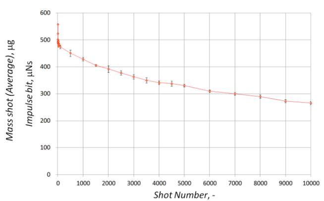
**Figure.13** Result of  $I_{bit}$  measurement
