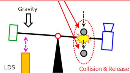
Figure.8 Method of  $I_{bit}$  calibration
