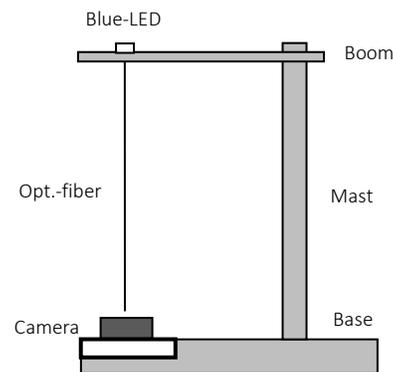
Fig. 2. Schematic of the DPVD.
