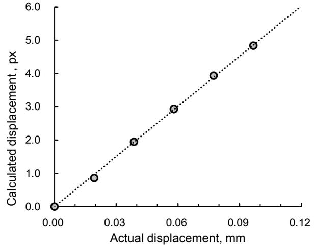
Fig. 5. Calculated vs. actual displacement.
