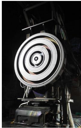
Fig 1. Left: The X3 thruster mounted on a thrust stand at UM. Right: Design goals of NASA's NextSTEP XR-100 project.
