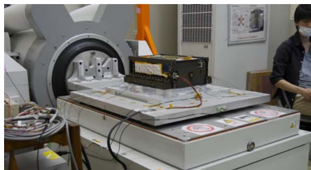
Figure 9. Configuration of EQUULEUS vibration test
