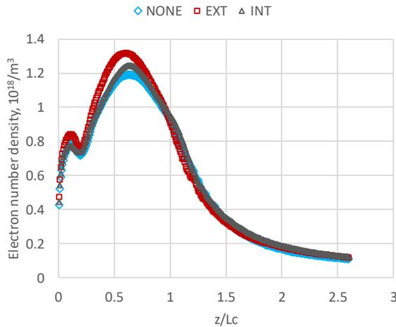
**Figure 4. Simulation result of electron number density on the channel center line.** Thruster anode is located at  $z/L_c=0$  and the channel exit is at  $z/L_c=1$ .
