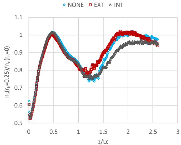
**Figure 5. Electron number at  $r_h=0.25$  relative to the channel center line.** The ratio is calculated at each  $z$  position.
