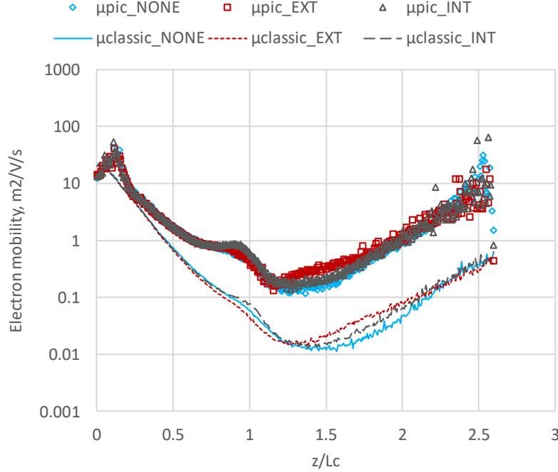
**Figure 6. Simulation result of electron mobility at  $r_h=0.25$ .** Lines show the electron mobility calculated according to the classical diffusion theory, whereas the symbols are the effective mobility as Eq. 5.
