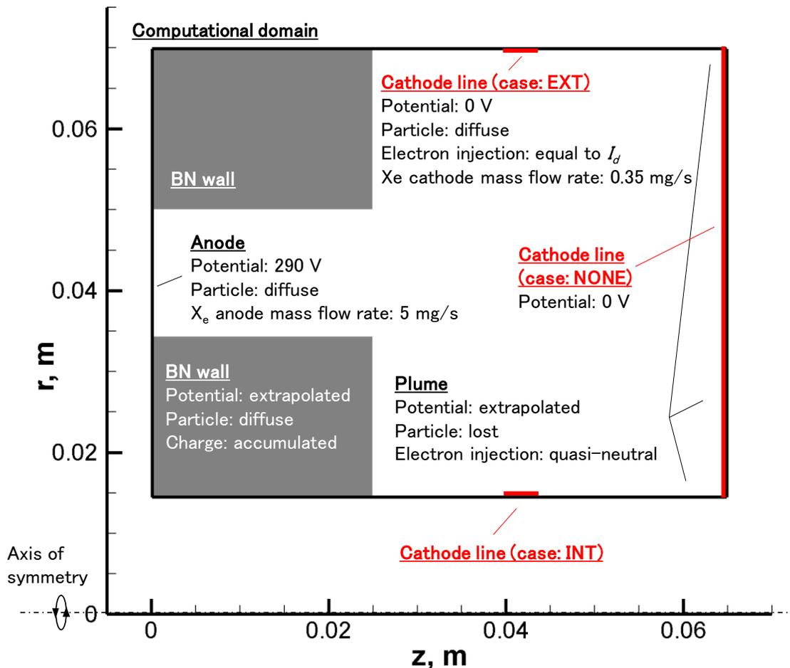
**Figure 1. Computational domain and setting of boundary conditions.** Three simulation cases were conducted for different cathode boundary placements: INT, EXT, and NONE. The potential of the right plume boundary was fixed to 0 V in the NONE case, whereas it was extrapolated with no gradient in other two cases.
