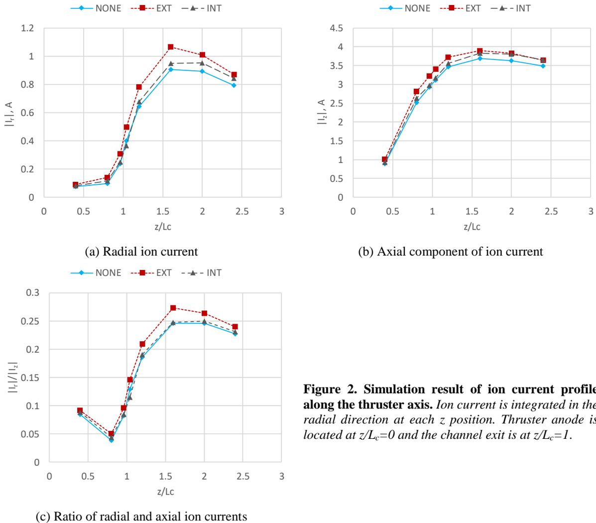
**Figure 2. Simulation result of ion current profile along the thruster axis. Ion current is integrated in the radial direction at each  $z$  position. Thruster anode is located at  $z/L_c=0$  and the channel exit is at  $z/L_c=1$ .**
