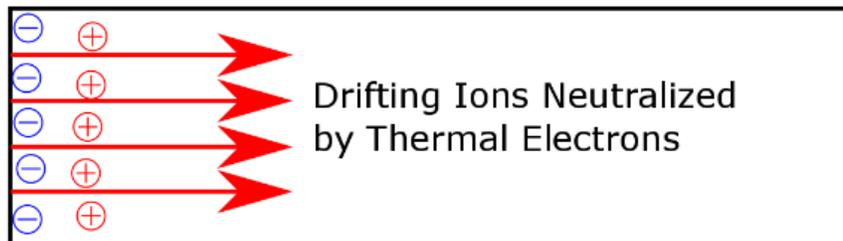
Figure 1. An idealized 1D ion beam neutralization model.
