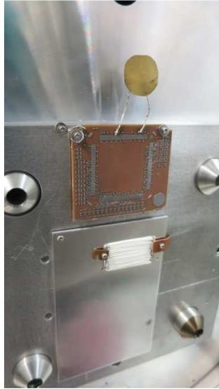
**Figure 7. View of the PCB and ETFE wires tested in the GEODUR test facility**
