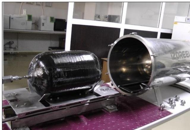
**Figure 7. Helium Leakage Test Setup**
