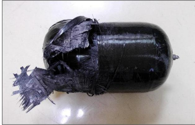
**Figure 8. Failure of XPT after Burst Test**
