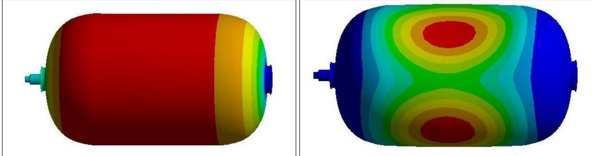
**Figure 3. XPT's First Axial and Lateral Modes**
