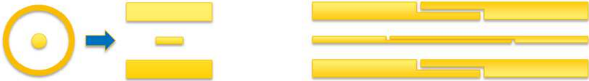
Figure 5: Left, a cross-section of a typical round coaxial waveguide compared to the rectangular cross section of a stripline; right, a side view of a conceptual finger joint showing the splitting of the stripline pieces into overlapping fingers.
