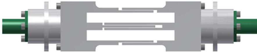
Figure 6: Side view of finger joint showing overlapping ground and center conductor plane to allow operation over a range from 0.7 - 2.5 GHz
