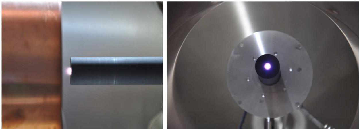
Figure 2: The high temperature testbed in operation with a C12A7 insert at the 150 mA and 5 sccm flowrate reported later in Figure 4.
