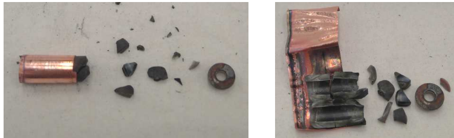
Figure 5: The C12A7 insert from the high temperature testing fractured and visibly degraded during the test. The piece at far right is the cathode orifice plate.
