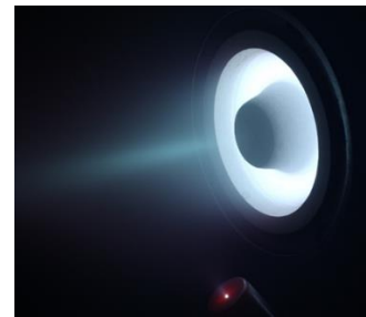
Figure 3. HT100 firing in SITAEL vacuum facility.
