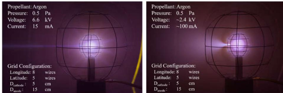
Figure 9. Tight jet (a) and spray jet (b) mode in IRS IEC.<sup>2</sup>
