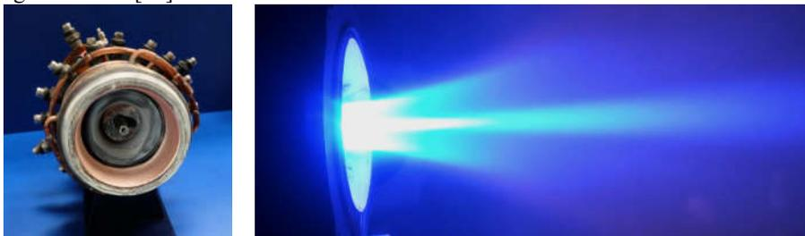
Fig. 3. Steady-state AF-MPD thruster SX3 thruster (left) in operation at 100 kW arc power, 690 A arc current, 400 mT of applied magnetic field and with argon mass flow rate of 120 mg/s.
