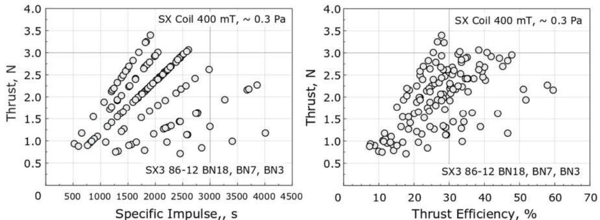
Fig. 4. Performance envelope of SX3 thruster at 400 mT.
