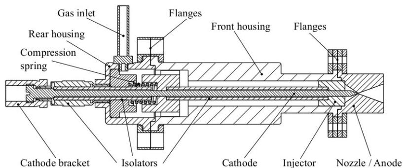
Figure 5. Schematic of the VELARC thruster.
