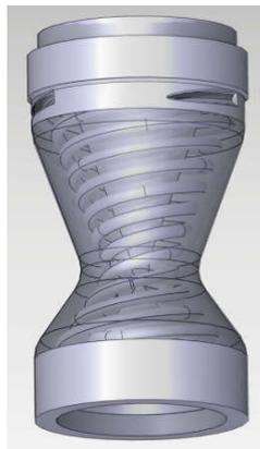
Figure 7. Design of a regeneratively cooled arcjet nozzle (ALM-based).
