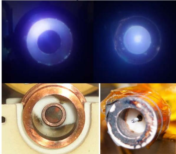
Figure 2: Upper left, PETRUS, upper right PETRUS2.0. Both operated at an energy of 5.12 J and at a voltage of 1600 V. Lower left and lower right both thrusters after 2072 pulses.
