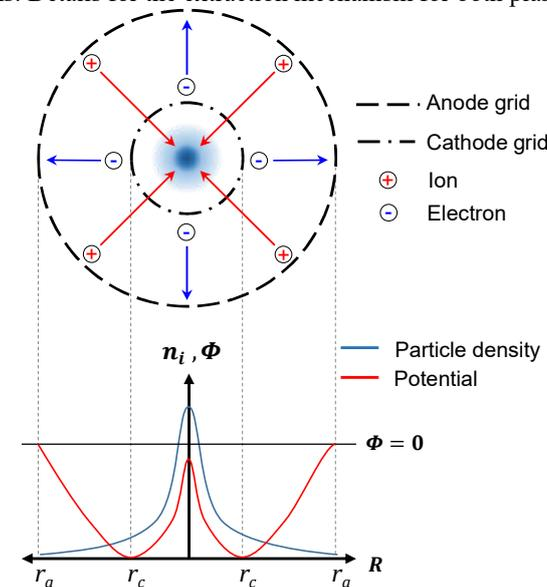
Figure 8. Schematic of IEC principle<sup>42</sup>
