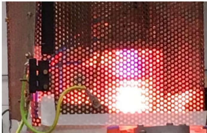
*Fig. 11 IPG6-S running on N<sub>2</sub> at 3.5 kW*
