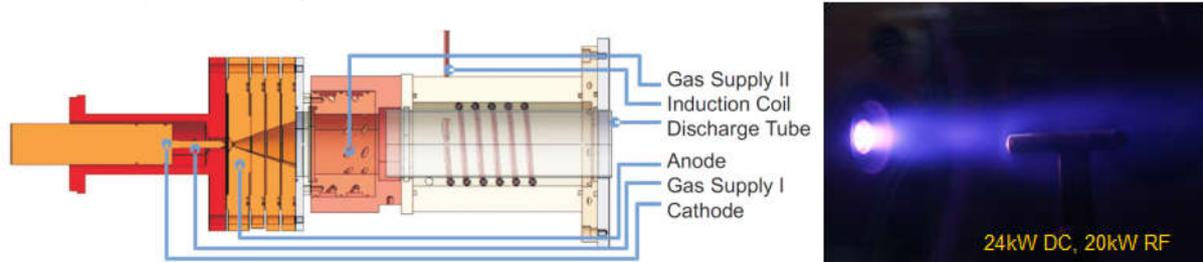
Fig. 12 TIHTUS schematic set-up and TIHTUS in operation (using IPG3 as second stage, hydrogen as propellant)
