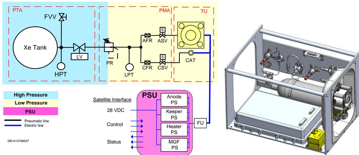
Figure 1. Left: System architecture of the LiteEPS. Right: CAD model of the LiteEPS
