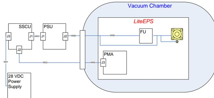
**Figure 3. Schematic of the experimental setup of phase II of the LiteEPS tests.**
