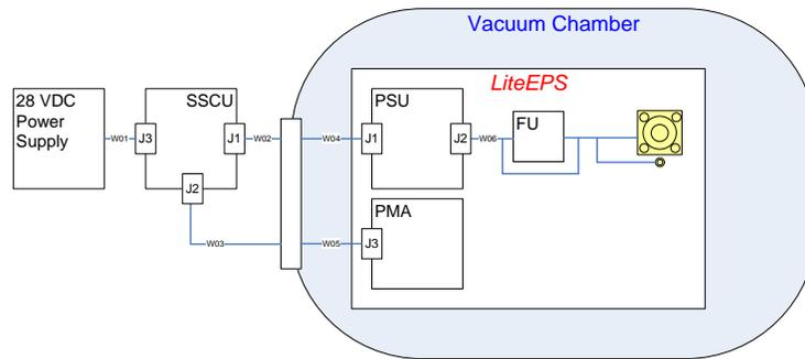
**Figure 4. Schematic of the experimental setup of phase III of the LiteEPS tests.**
