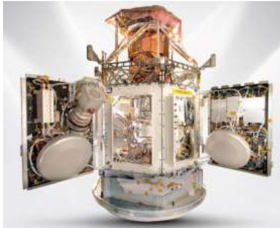
Figure 4. Venus satellite internal view
