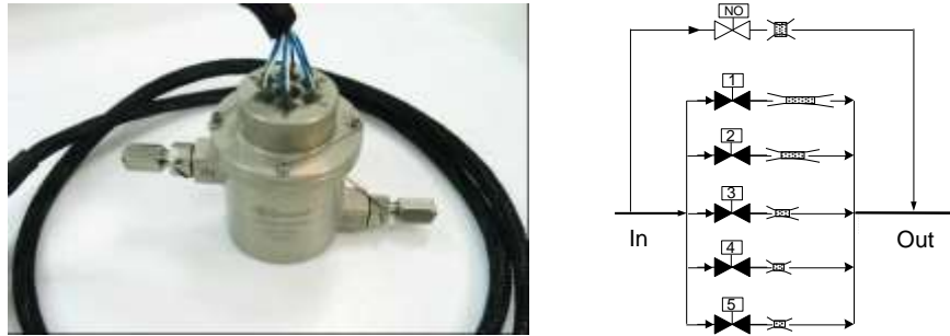
Figure 11. Controller (DXFC): flight model (left) and block diagram (right)
