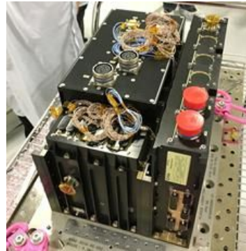
Figure 9 - Elektro PPU EQM with its instrumentation
