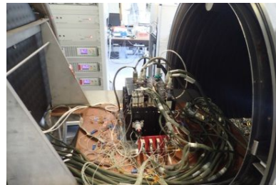
Figure 10 - Elektro PPU EQM in the thermal chamber
