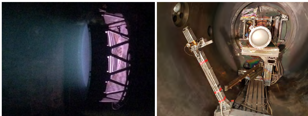
Figure 3. Photograph of RIT 2X operating in a vacuum test facility and part of the beam diagnostics setup.
