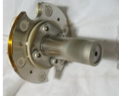
Fig. 2 Photo of developed thermionic emission type hollow cathode with LaB 6 emitter.
