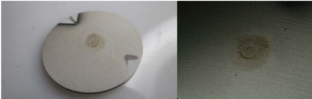
Figure 7. Synergetic erosion evidences – pictures of the sample M26 after 35 hours of irradiation
