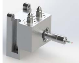
Figure 5. Rendering of the cathode and anode module that supports a single thruster.
