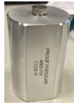
Figure 10. Breadboard crush seal test unit
