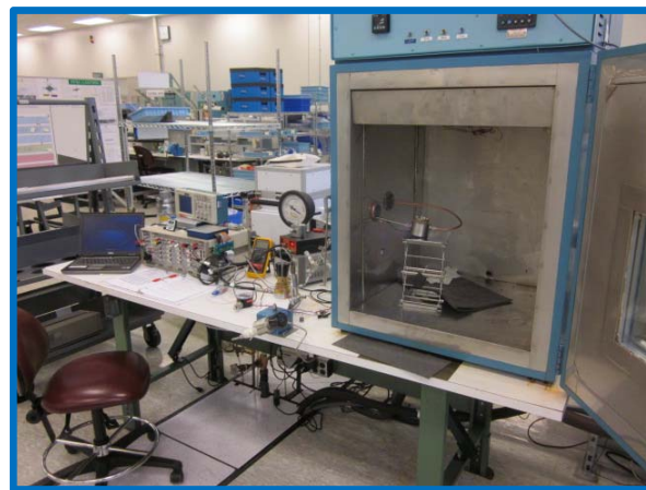
Figure 4. Steady State flow test set-up
